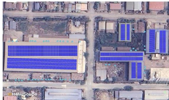
**Figure 6.** Rooftop PV Design Layout for Group 4
