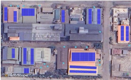
**Figure 5.** Rooftop PV Design Layout for Group 3
