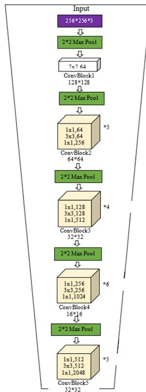
**Figure 9.** ResNet50 as Encoder of Unet
