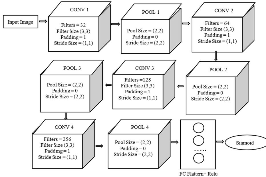
**Figure 3.** Block Diagram of Custom CNN Model
