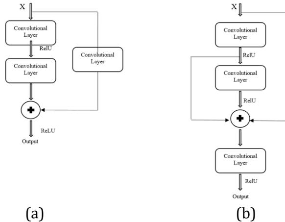
**Figure 6.** (a) Residual Block (b) Dense Block
